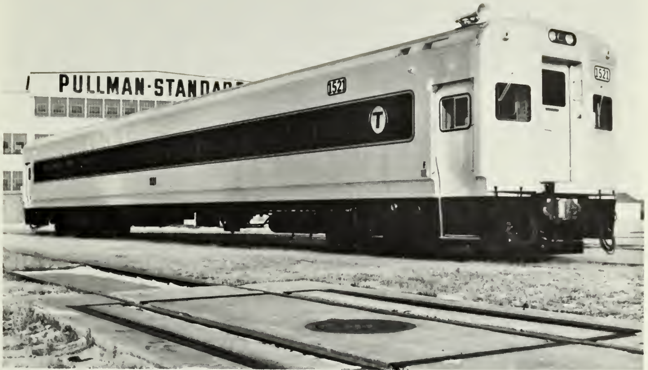
ALUMINUM-CLAD COACH is one of 25 Pullman Standard will manufacture for MBTA commuter railroad service under a contract signed December 7.
